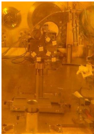
Figure 2: Experimental autoclave inside the hot cell.
