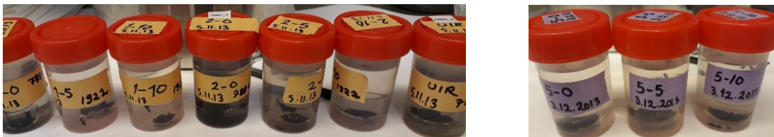
Figure 2: The old samples, 233 U alpha doped UO 2 fragments placed in glass saucers inside the test vessels during the bicarbonate pre-leaching without iron.
